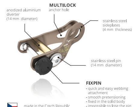
Paddle is an anchoring device for 50 mm wide webbing. It is designed to anchor tricklines up to 14 kN tension. Locking mechanism allows to pretension webbing in one way, whilst it is fixed in the other way. Paddle has smooth edges, so there is no danger of destroying the webbing. Thanks to middle axis with 26 mm diameter, the webbing retains more than 85% of its strength. Paddle FX can be attached to the anchor by most of available connectors (shackles, quicklinks etc.).
