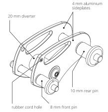
MITHRIL is a 25 mm webbing anchoring device designed for usage with a soft release. That means the rear pin must be always loaded only in 1 axis - the center line between both sideplates. Triloading deacreases strength of
